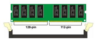
Please check the pin number to match the socket side well before installing memory module.
